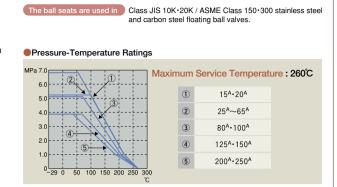
The ball seats are used in Class ASME Class 150·300 stainless steel and carbon
